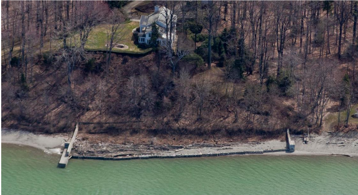
Figure 6.24: Concrete and concrete-cube groyne pair with low connecting seawall near Avonia Beach, western Erie County. This approach cordons off the natural beach from fair-weather wave attack that is often beneficial (April 2015 imagery, available from PA DEP Coastal Resources Management Program at http://www.dep.pa.gov ).
