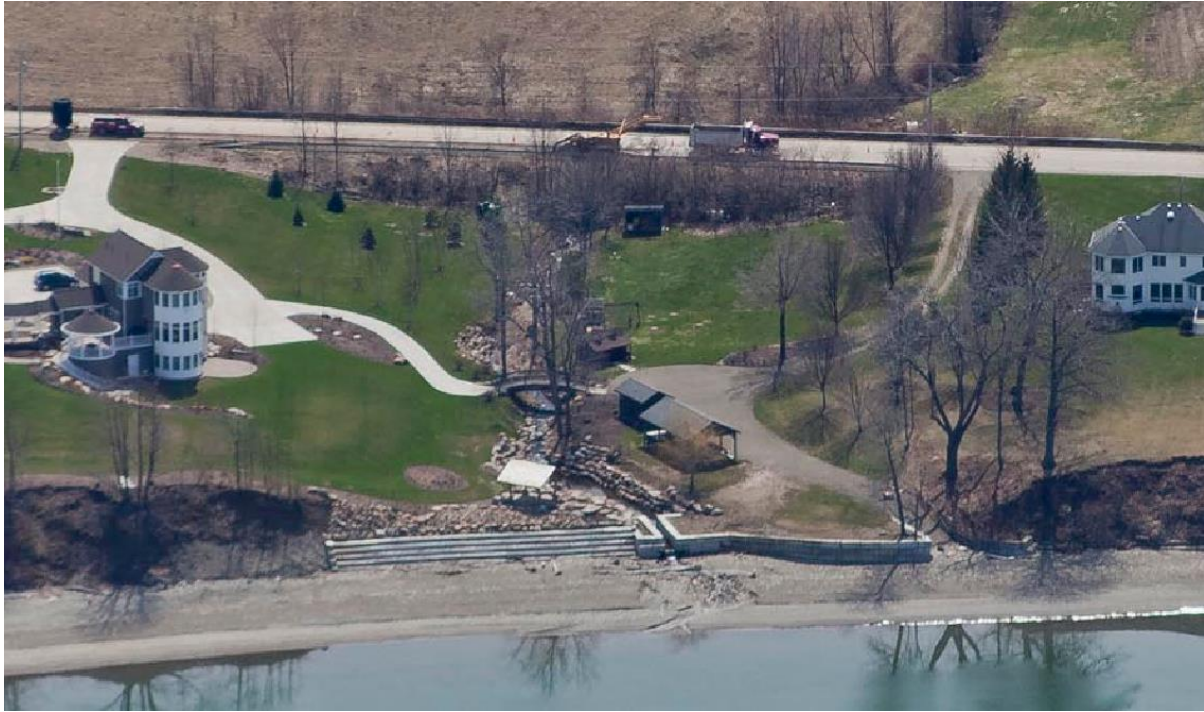
Figure 6.12: Stepped concrete revetment and back-filled concrete-cube seawall (bulkhead) in easternmost Erie County. A bedrock toe is absent at this location (April 2015 imagery, available from PA DEP Coastal Resources Management Program at http://www.dep.pa.gov ).
