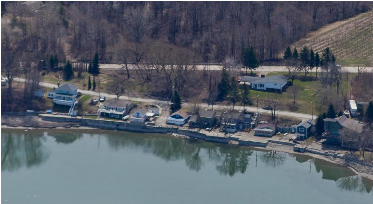
Figure 6.13: Back-filled concrete-cube bulkheads protect properties built on a low bank east of Twentymile Creek, eastern Erie County (April 2015 imagery, available from PA DEP Coastal Resources Management Program at http://www.dep.pa.gov ).
