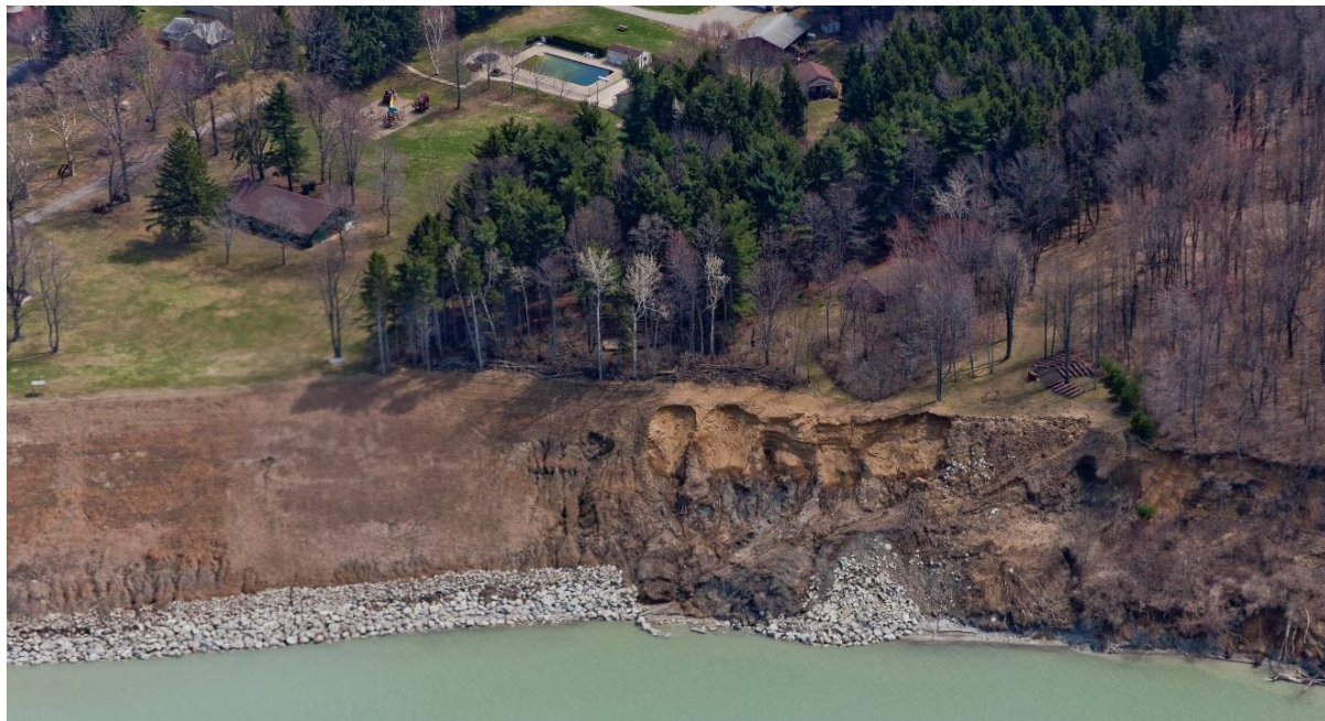
Figure 6.1: Bluff failure in western Erie County (right side of image). Small rotational slumps occur in lacustrine sediments near the top of the bluff, while debris slides and soil creep occur in glacial tills on the lower bluff. Nearby erosion-mitigation efforts (on the left) include slope re-grading and placement of riprap at the bluff toe (Imagery collected in April 2015 and is available from PA DEP Coastal Resources Management Program at http://www.dep.pa.gov ).
