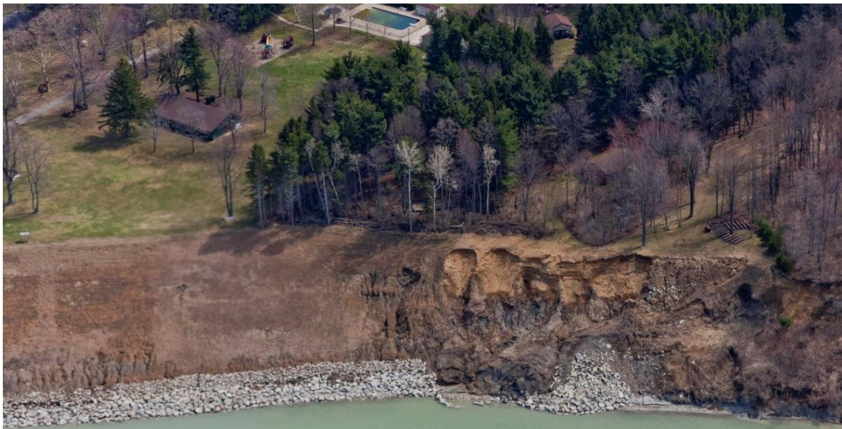
Figure 3.4: Typical appearance of bluff failure along high bluffs in western Erie County. Small rotational slumps occur in lacustrine sands at the top of the bluff; and debris slides occur in glacial tills in the lower half. The bedrock toe is absent. Erosion-mitigation efforts (left side) involve slope re-grading and placement of rip-rap at the bluff toe (Imagery collected in April 2015 and available from Pennsylvania DEP Coastal Resources Management Program at http://www.dep.pa.gov ).
