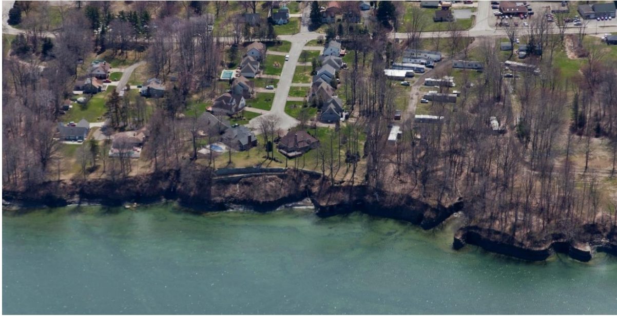
Figure 3.3: Typical appearance of coastal bluffs in western Harborcreek Township. Pronounced irregularities in the bluff crest trend are caused by preferential erosion at joints and faults in the Devonian Bedrock. Bedrock makes up the lower ~50% of these low bluffs that are capped by glacial till (Knuth and Lindenberg, 1995). In the nearshore, larger fault/joint traces trend towards the “4:30” and “7:30” clock positions (Imagery collected in April 2015 and available from Pennsylvania DEP Coastal Resources Management Program at http://www.dep.pa.gov ).
