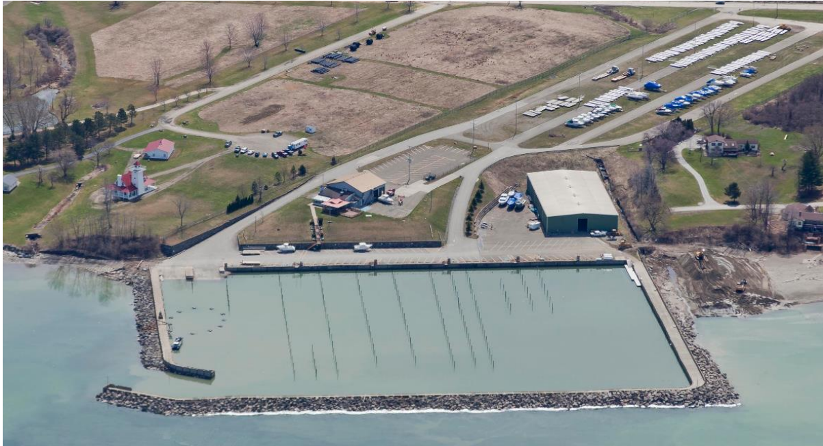
Figure 6.14: Shore-attached breakwaters and low banks at North East Marina, eastern Erie County. Bedrock is below lake level at this location. Artificial sediment bypassing is in progress on the updrift (right) side of the marina and will be moved to the downdrift (left) side (April 2015 imagery, available from PA DEP Coastal Resources Management Program at http://www.dep.pa.gov ).
