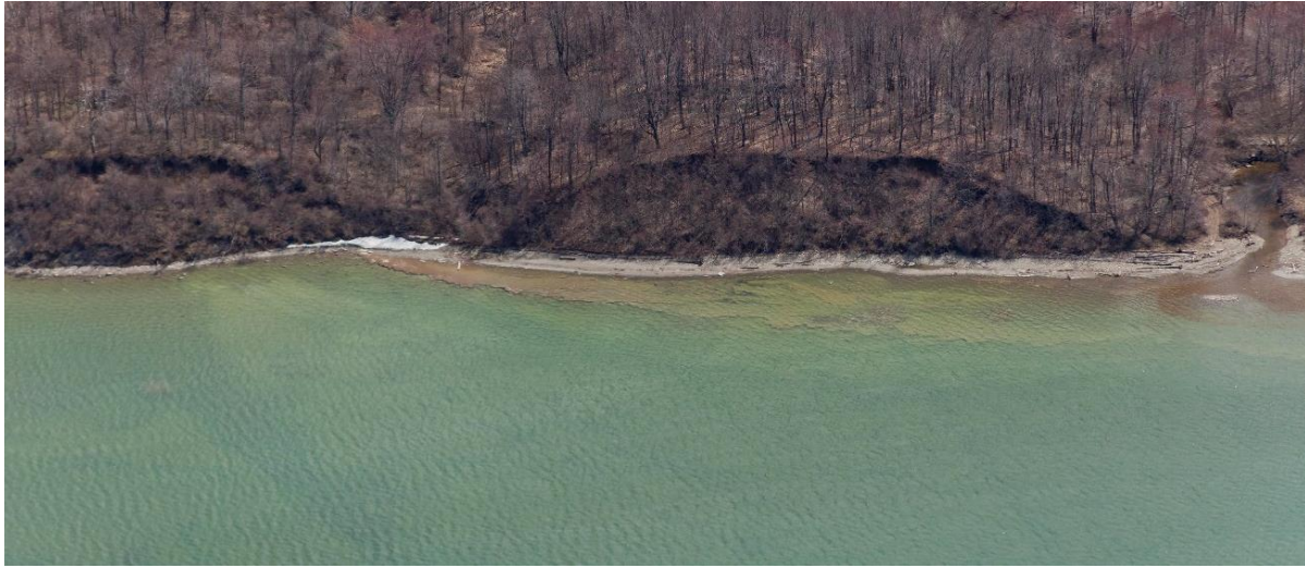
Figure 3.6: Typical appearance of coastal bluffs in western Erie County, just east of Conneaut, OH. A Devonian bedrock toe is absent in this area, but shale crops out on the lake bed below lake level in the foreground. Two large faults or fractures cross the nearshore bedrock surface (dark linear features) which indicates minimal nearshore sediment coverage. The features extend lakeward of the bluff face, trending towards the “4:30” clock position (Imagery collected in April 2015 and available from Pennsylvania DEP Coastal Resources Management Program at http://www.dep.pa.gov ).
