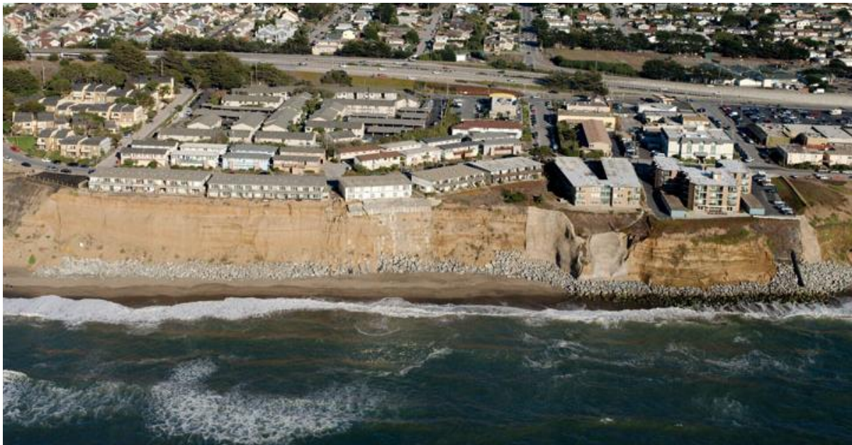
Figure 6.8B: Oblique aerial photograph (from 2013) of the Esplanade Apartments complex, Pacifica, California. By early 2016, two of these complexes had been condemned and demolished because bluff erosion had undermined the buildings. The addition of extra riprap, concrete grouting and bluff face-anchoring did not prevent continued bluff retreat (Images: modified from an aerial photo database available from the California Coastal Records Project at Californiacoastline.org ).
