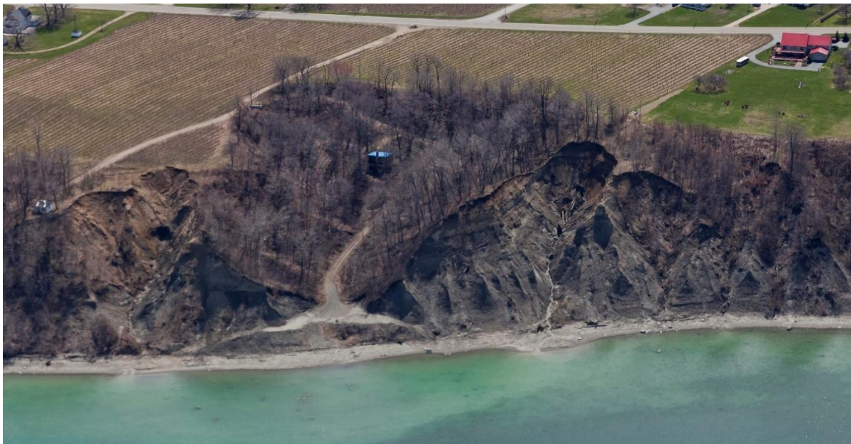
Figure 3.7: Oblique aerial photo showing the typical appearance and stratigraphy of eroding high bluffs in eastern Erie County near North East (and near the location of Figure 3.5). Curved and sharp bluff edges at the headwall scarps of four active rotational slumps can be seen on either side of a large vegetated Holocene bowl that contains a blue-roofed building and a beach-access trail. Note the spring-fed stream exiting the active slump to the west of the beach-access trail. It is sourced by groundwater from the unconfined aquifer in the upper lacustrine/beach-ridge section of the bluff (tan colored). Glacial tills (grey color) occupy the lower two-thirds of the bluff. The flat plateau inland of the bluffs is part of the beach-ridge complex associated with the Warren paleoshoreline (Imagery collected in April 2015 and available from the Pennsylvania DEP Coastal Resources Management Program at http://www.dep.pa.gov ).
