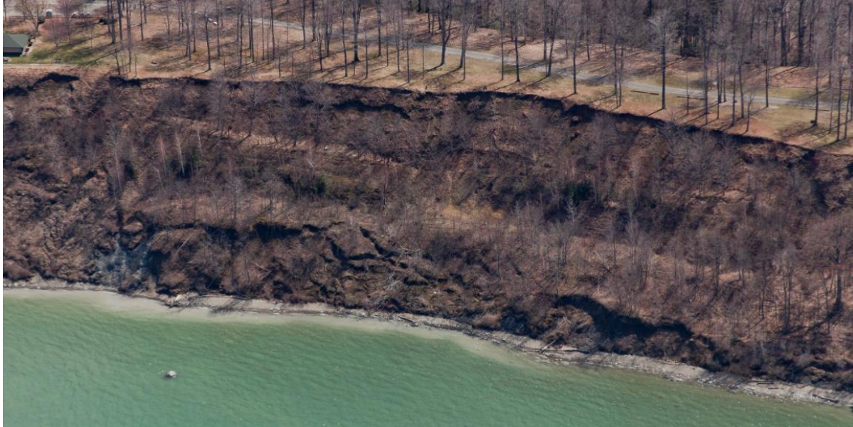
Figure 3.10: Oblique aerial photo showing a translational slump (slide) with a relatively linear bluff-crest headwall. The failure is developed in bluffs consisting of glacial tills and overlying lacustrine sands in western Erie County. Three sloping headwall scarps and two intervening sub-horizontal benches are visible. The lowermost headwall scarp at the shoreline also shows more recent earth flow and soil creep activity (Imagery collected in April 2015 and available from the Pennsylvania DEP Coastal Resources Management Program at http://www.dep.pa.gov ).
