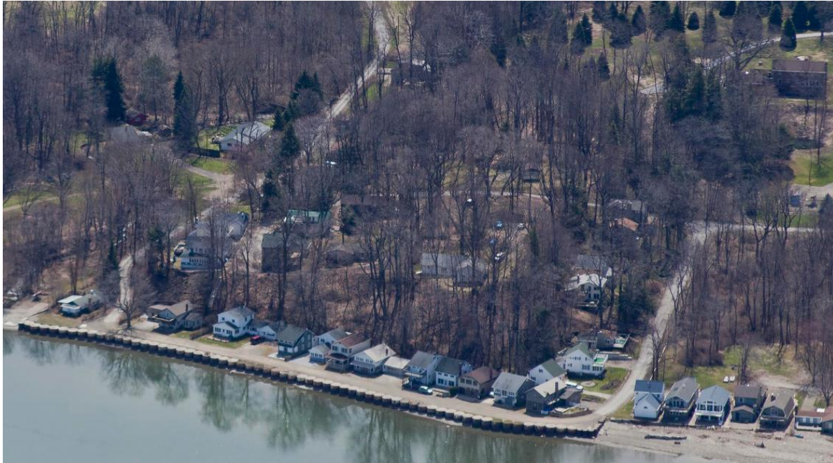
Figure 6.16: Concrete filled caissons with backfill protect buildings along a low coastal bank east of Freeport Beach at Sixteenmile Creek, eastern Erie County (April 2015 imagery, available from PA DEP Coastal Resources Management Program at http://www.dep.pa.gov ).
