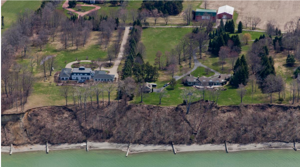
Figure 6.22: Small non-parallel groyne field in western Erie County. Beach accumulation between the groynes keeps wave energy away from bluff at these two properties (April 2015 imagery, available from PA DEP Coastal Resources Management Program at http://www.dep.pa.gov ).
