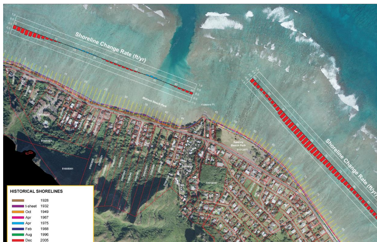
Figure 7.1: Screenshot of a section of the Oahu, Hawaii, coast showing a typical map product generated by DSAS in GIS. On this non-bluff coast, changes in the low-water shoreline are tracked over time (1928 to 2005; various data sources). Virtual monitoring transects are shown in yellow, historical shorelines by variously colored line features, and coastal-change summaries by bar graph (red is erosion; blue is accretion; maximum erosion rate \sim 0.24 m/year) (Hawaiian coastal data from ftp://soest.hawaii.edu/coastal/webftp/Oahu/posters/KaaawaSTsmoothTMKPosterRGB72.jpg ).
