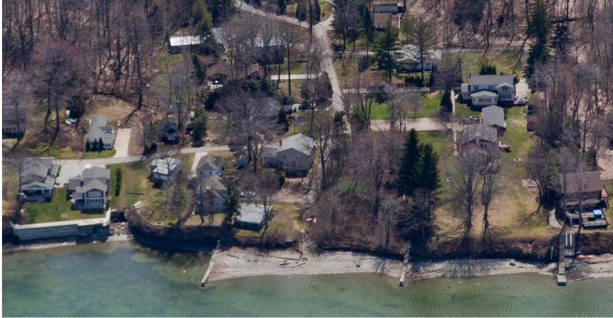
Figure 6.20: Concrete-cube bulkheads and groynes west of Eightmile Creek, eastern Erie County. Trapping of littoral sand by groynes removes the focus of wave attack from the low bluff (with a steep bedrock-toe) on the updrift sides of the structures (April 2015 imagery, available from PA DEP Coastal Resources Management Program at http://www.dep.pa.gov ).
