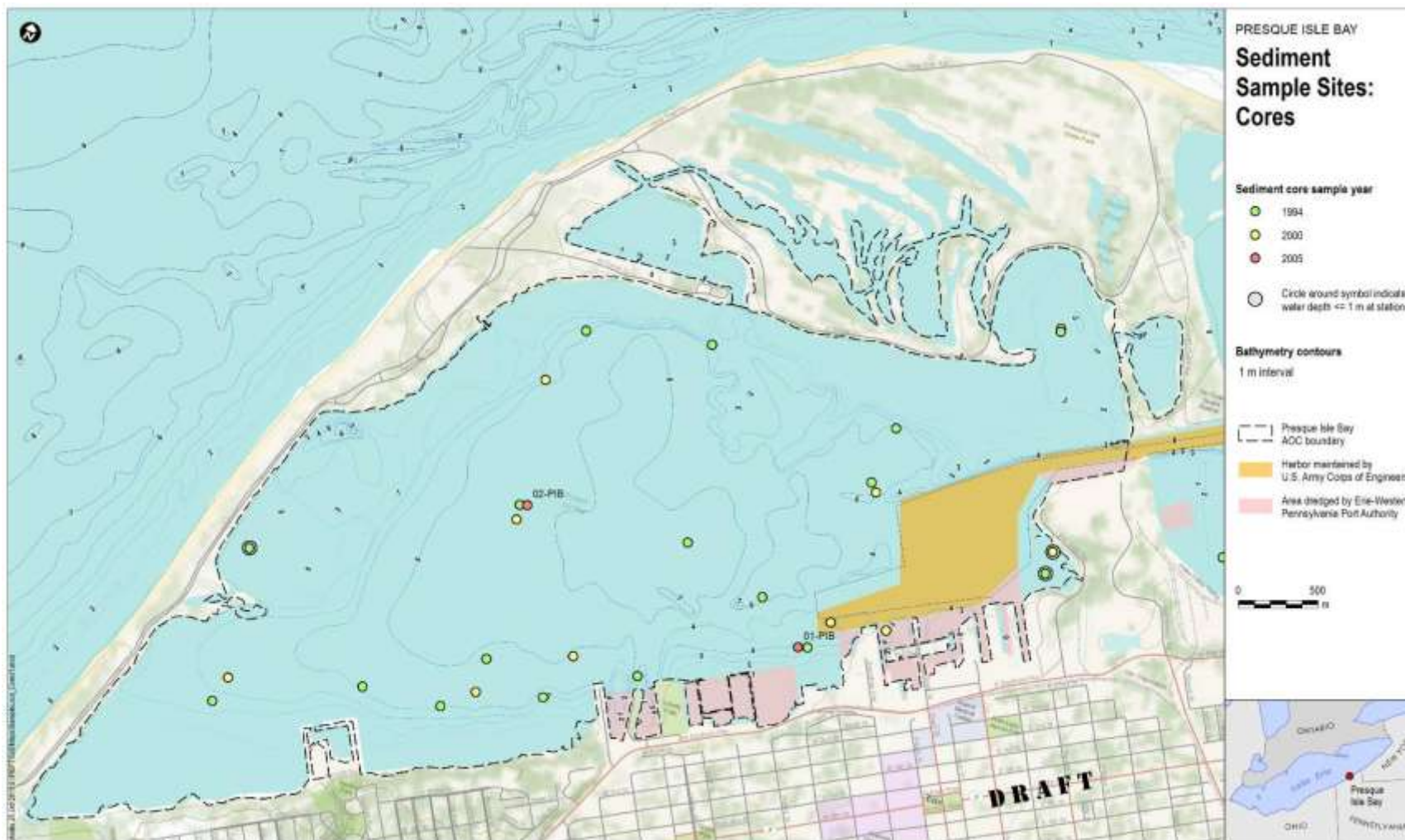
Figure 3.2 Core sediment sampling locations performed in PIB
