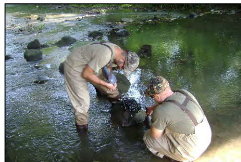
Figure 10. Staff assessing pH, temperature, conductivity, and DO in Conneaut Creek
