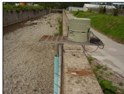
Figure 8. ISCO 6712 sampler used to collect storm water from Mill Creek
